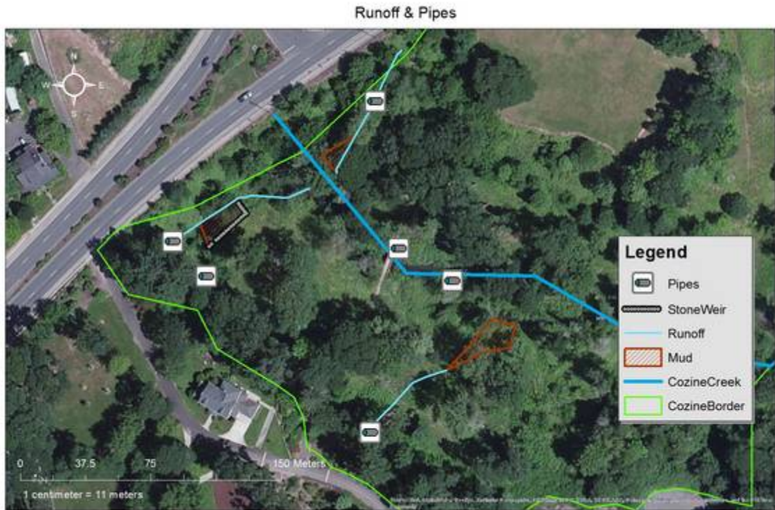
Figure 6: The location of pipes and the paths runoff follows. Other factors that affect runoff, including weirs and mud fields are also shown.
