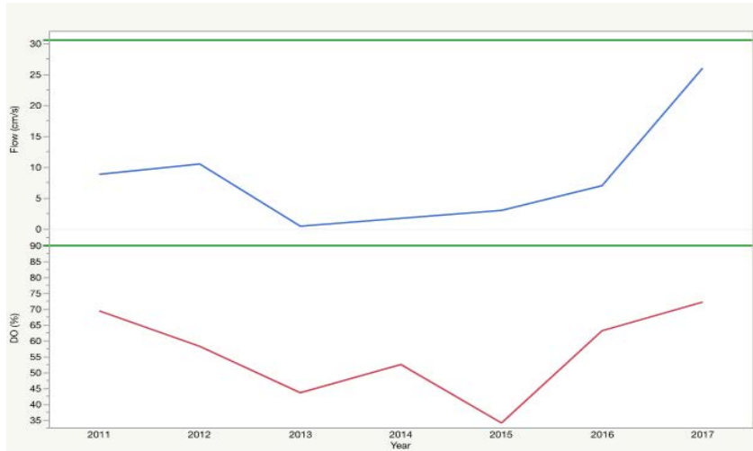
Figure 12. Comparing trends for mean dissolved oxygen and flow rates from 2011 to 2017 at the Linfield College site. The green lines represent ideal values or ranges for salmon (90% and 30.48 cm/s) (Wasowski et al. 2013; Riley et al. 2009).
