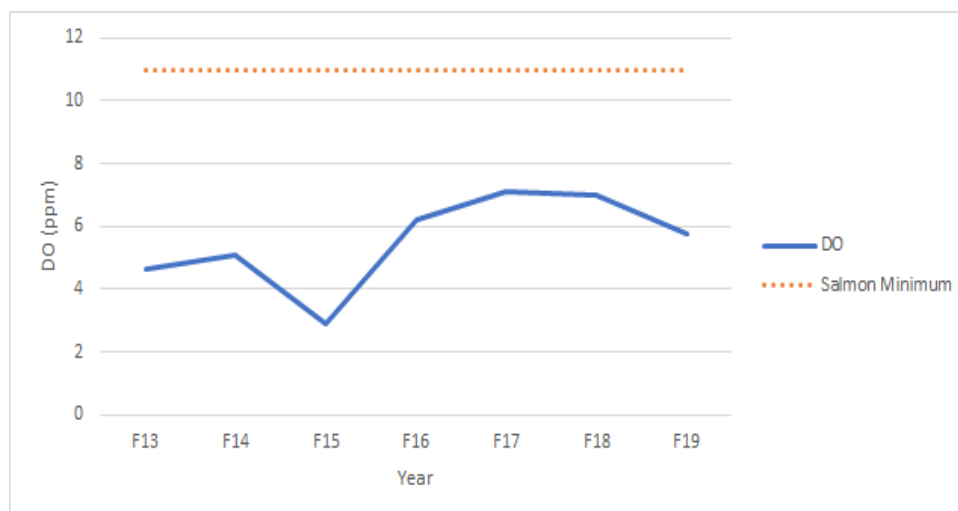
Figure 13. Mean dissolved oxygen (ppm) at the Linfield College site in fall 2013 to 2019. The dotted line represents the acceptable minimum DO (ppm) level for salmon at 11 ppm (Kidd, 2011).
